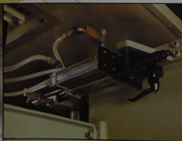
The hydraulic control for the cutter head infeed for centre station work. This provides smoother entry into the workpiece when starting the table.
