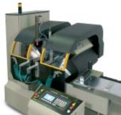
The particular structure allows both DH 500 A and DH 550 A to perform a min cut of 320 mm with both tilted heads at 45°
